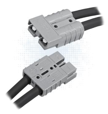
Based off the design pioneered by Anderson in 1953, APP®'s two pole SB® connectors set the standard for DC power distribution and battery connections. SB®50 connectors feature a one piece plastic housing using stainless steel springs to hold low resistance contacts in place. Wires sizes from #16 (1.5 mm²) to #6 (13.3 mm²) are held in the smallest of the SB® series housings.
