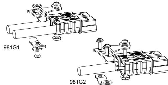
The given wire O.D. information is an estimate. Cable clamps should be evaluated for performance with the actual wire to be used.
