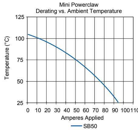
NOTE: Temperature rise charts are based on a 25°C ambient temperature. Powerclaw charts are based on #8 AWG equivalent copper foil on board side, mated to #6 AWG conductor on wire side.
