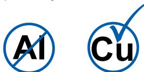
APP® connectors are designed to be crimped and/or soldered to multi-stranded copper conductor wires only. Alternate conductor materials including aluminum should not be used. Aluminum conductors crimped into APP® contacts can result in a galvanic reaction occurring between the aluminum wire and the more cathodic metals used in APP® contacts including copper, tin, silver, and gold. Additionally softer metals like aluminum flow or loosen from crimps much easier than copper.
