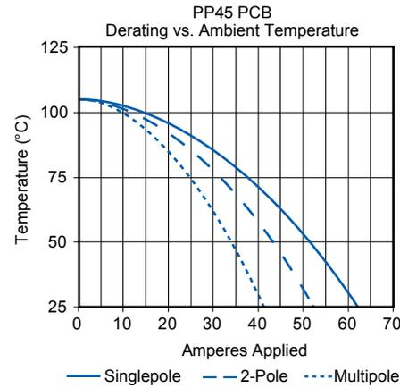
NOTE: Temperature rise charts are based on a 25°C ambient temperature. PP25 PCB charts based on 0.002 in<sup>2</sup> foil on board side, mated to #12 AWG conductor on wire side. PP45 PCB charts based on #10 AWG equivalent copper foil on board side, mated to #10 AWG conductor on wire side.
