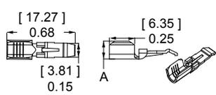
K\* - For #10 AWG class K stranded wire or smaller. For larger wires use superflex contacts.
