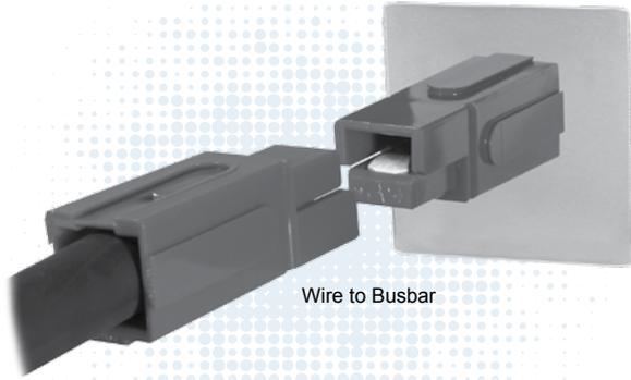
PP180 are the largest of the Powerpole® series housings. They are designed to accommodate up to 3/0 (70 mm<sup>2</sup>) wires and handle high currents up to 350 amps. Busbar contacts are also available for power inputs and takeoffs. Color-coded housings minimize user confusion and the potential of cross mating circuits.
