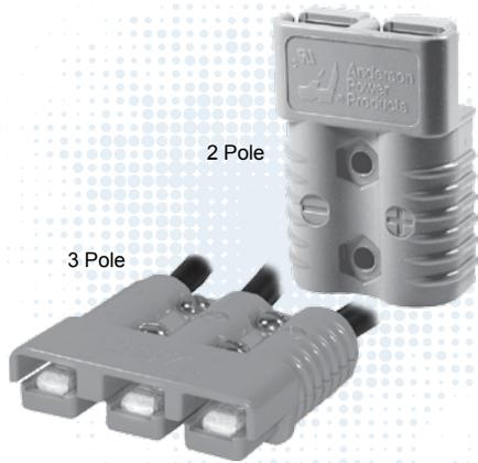
Wires sizes from #12 (3.3 mm<sup>2</sup>) to 1/0 (50 mm<sup>2</sup>) fit in the second to largest connector in the SB® series. The 3 pole SB®175 adds an additional position for power or grounding. All Multipole wire connector housings are genderless and mate to themselves minimizing inventory and assembly complexity.
