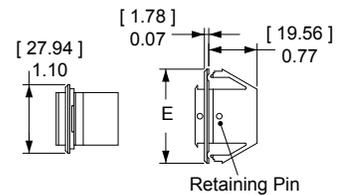
NOTE: Retaining pins are used to secure and position Powerpoles® in one of two positions in receptacle shells.
