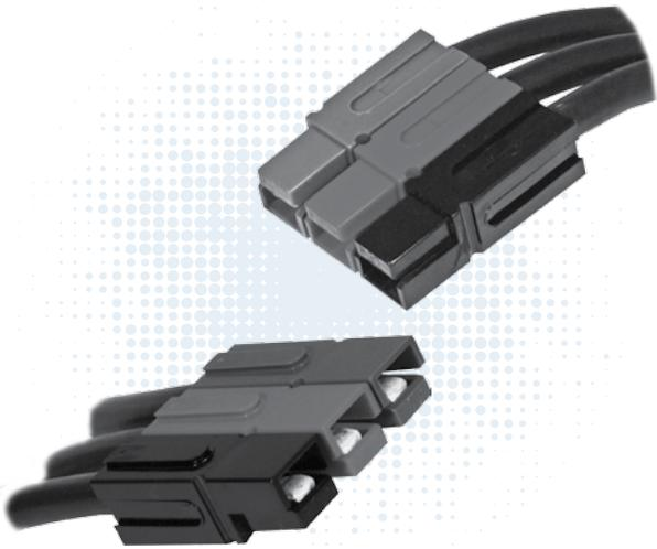
PP120 series Powerpole® housings are designed to accommodate up to 1/0 (50 mm<sup>2</sup>) wires and handle high currents up to 240 amps. Reducing bushings allow PP120 to accept down to #8 (10 mm<sup>2</sup>) wires. Multiple colors of stackable housings combine with APP®'s low resistance flat wiping technology to offer powerful connection capability.
