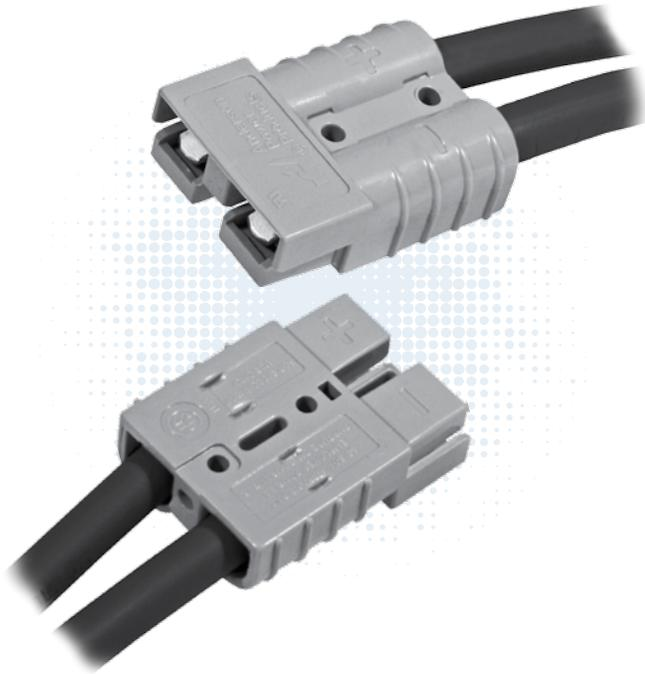
Based off the design pioneered by Anderson in 1953, APP's two pole SB® connectors set the standard for DC power distribution and battery connections. SB®50 connectors feature a one piece plastic housing using stainless steel springs to hold low resistance contacts in place. Wires sizes from #16 (1.5 mm<sup>2</sup>) to #6 (13.3 mm<sup>2</sup>) are held in the smallest of the SB® series housings.
