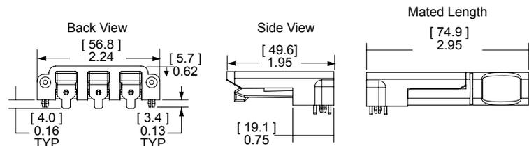
See PCB connector drawing on website for further detail.
