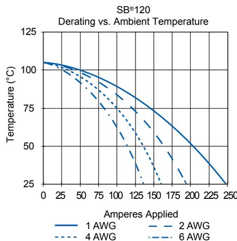
NOTE: Temperature rise charts are based on a 25°C ambient temperature.
