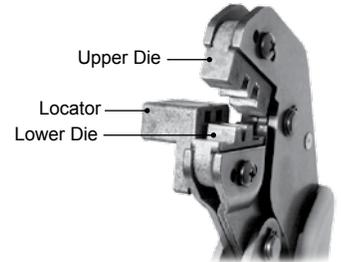
**1309G3:** For crimping PP15/45 loose piece strip contacts from #10 – 16 AWG (5.3 – 1.3 mm<sup>2</sup>)
