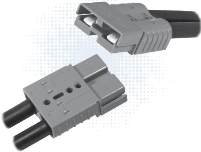
Like the other Multipole connectors, the SB<sup>®</sup>120 offers color-coded mechanically keyed housings. Keys can be used to identify and separate different circuits, or prevent users from accidentally cross mating different voltages. Wires sizes from #10 (5.3 mm<sup>2</sup>) to #1 (42.4 mm<sup>2</sup>) are held in the second smallest SB<sup>®</sup> housing.
