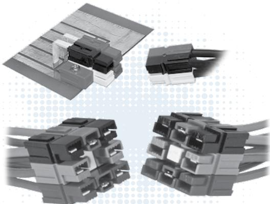
PP15-45 series are the smallest Powerpole® housings. They can be used for wire-to-wire or wire-to-board applications. Wire sizes from #20 AWG (0.5 mm<sup>2</sup>) to #10 (6 mm<sup>2</sup>) offer power capabilities up to 55 amps per pole. Finger proof housings and the ability to incorporate first-mate last-break ground connectors enhance the capabilities of this Powerpole® series.
