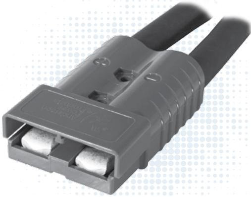
The SB®350 is the largest connector in the series with power capabilities up to 450 amps with 4/0 wire. Wires ranging from #1/0 (50 mm<sup>2</sup>) to 300 mcm (152 mm<sup>2</sup>) fit into the one piece housing available in standard PC or a chemical resistant PBT/PC blend. Silver plated wire or busbar contacts minimize electrical resistance while offering supreme durability and reliability.
